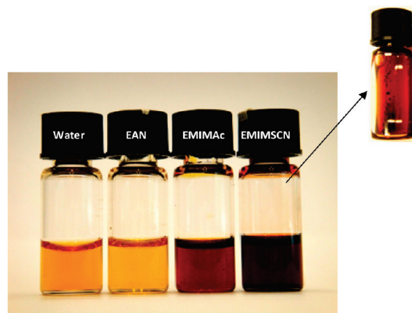
Figure 4. Dilute, polymer-coated maghemite dispersions in various solvents.
